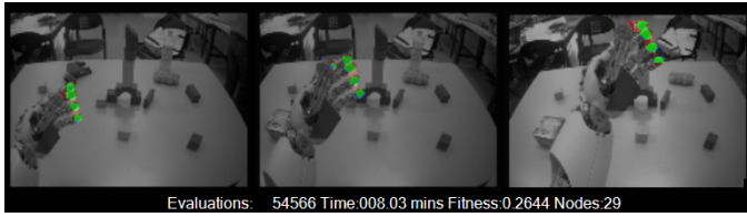
Fig. 7. Results when visually locating the fingertips of the iCub .
