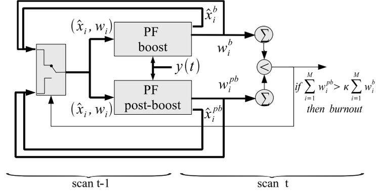
Figure 4: Burnout detection algorithm
