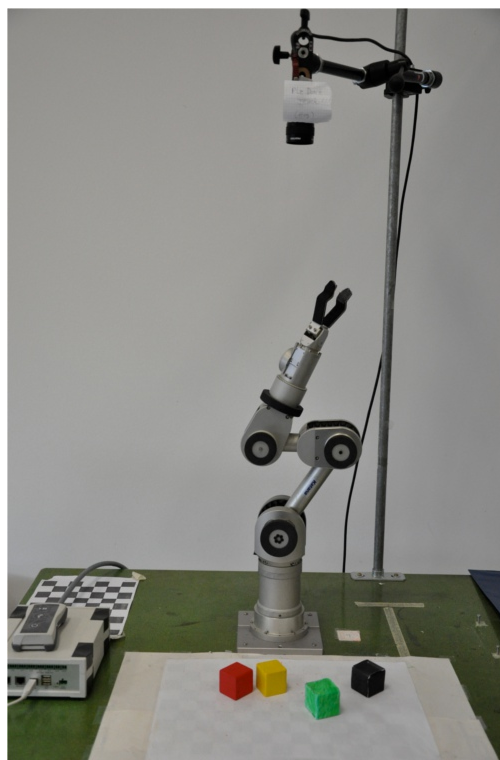
Fig. 1. The Katana robot arm in its block-world environment. It reaches for, grasps, and places blocks. The sensory input is an image from the overhead camera. There is a Markov Decision Process environment representation (discrete states and actions). Reinforcement learning updates a policy for action selection. The only reward is intrinsic: learning progress of a set of predictors (one for each state) that predict the outcome of that action. At any time, it prefers to try the state-action pairs that are associated with higher progress.
