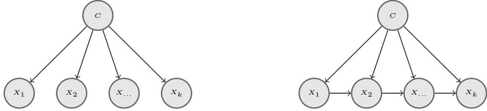
Figure 6: Structure of naive Bayes (left panel) and TAN (right panel). The TAN structure contains the same arcs of naive Bayes, with an additional tree that connects the features.
