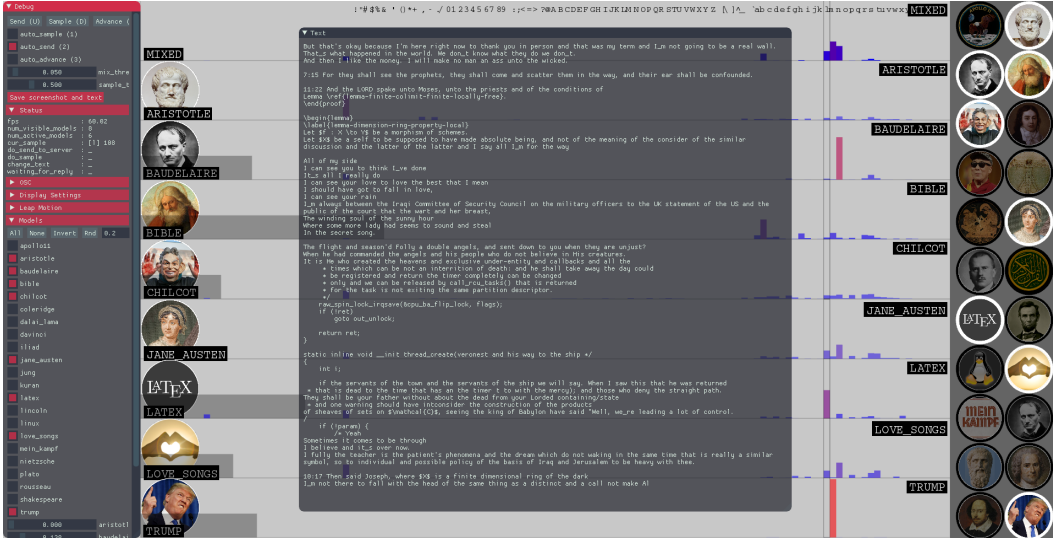
Figure 1: Example screen output and generated text. The user can select multiple models with over 20 to choose from. The chosen models are instantly available to interact with. The blue-red vertical bars visualise the probability distributions at the current time-step t , one row per active model ( y_t^i for the i 'th model), and the mixed probability distribution \rho_t (the top row). The horizontal dark grey bars on each row visualise the mixture weights for each model, stored in the vector \pi_t .
