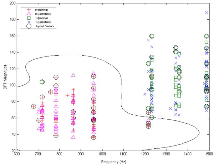
Figure 7. Detection rate of low and high DTMF frequency groups for  $\alpha = 1.2$
