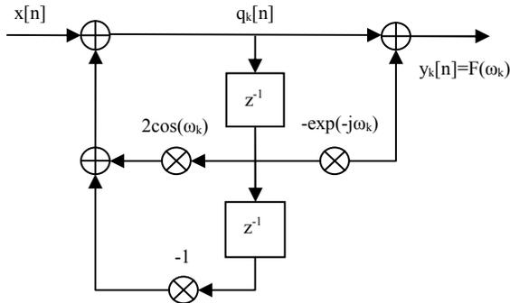
Figure 1. Block diagram of Goertzel's Algorithm
