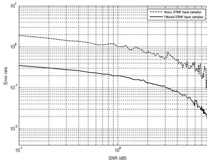
Figure 8. SNR vs. error rate for noisy and filtered DTMF input samples
