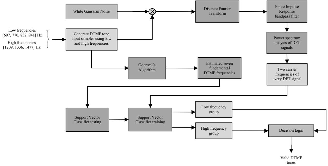
Figure 2. Proposed hybrid DTMF tone detection model
