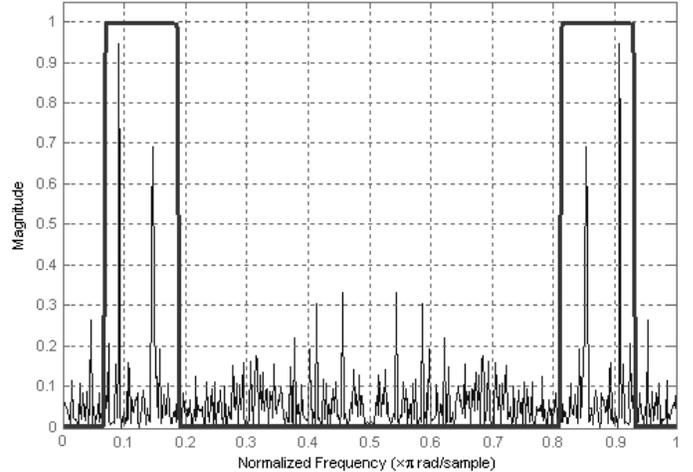
Figure 3. FIR bandpass filter applied to power spectrum of DTMF signal corrupted with noise coefficient  $\alpha = 0.5$
