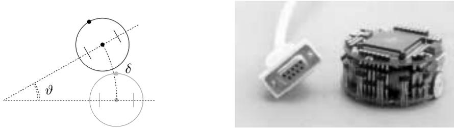
Figure 3: Displacement values for the robot (left side), the Khepera robot (right).
