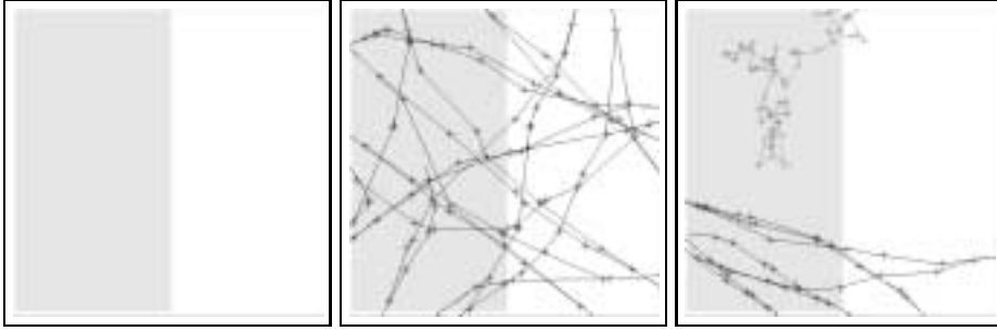
Fig. 1. (Left) The squared arena and the “half-full” Region : I = 0.49 . The arena side is 500 unit long. (Middle) Trajectory of one Ibot running a solitary trial with N_{max} = 100 and Prog = (30^\circ, 200) . Crosses indicate sampled points. The result is N_{in} = 52 , \hat{I} = 0.52 . (Right) Trajectories of two Ibots running a shared trial with N_{max} = 100 , starting from a scattered configuration and running private control programs: Prog^1 = (180^\circ, 50) (gray trace), Prog^2 = (20^\circ, 150) (black trace). The result is N_{in}^1 = 55 , N_{in}^2 = 30 , \hat{I} = 0.85 . Ibot 1 took N_{sam}^1 = 61 samples, Ibot 2 took N_{sam}^2 = 39 .
