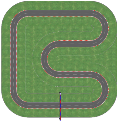
Figure 6: Training race track. The controllers were evolved using a track of length of 714.16m and width of 10m, that consists of straight segments of length 50 and 100m and curves with a radius of 25m. The car starts at the bottom (start line) and has to drive counter-clockwise. The distance from the edge of track to the boundary guardrail is 14m.
