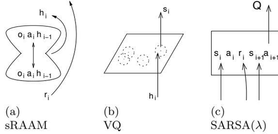
Fig. 2: SERVO. The sRAAM autoencoder is trained using back-propagation on  $\mathbf{p}_i \oplus \mathbf{h}_{i-1}$ . After training  $\mathbf{h}_i$  is generated using  $E$  and is passed the internal state layer. VQ assigns an internal state  $\mathbf{s}_i$  to the representation  $\mathbf{h}_i$  of the history. The RL layer receives Markovian data and learns an action-value function using SARSA( $\lambda$ ).
