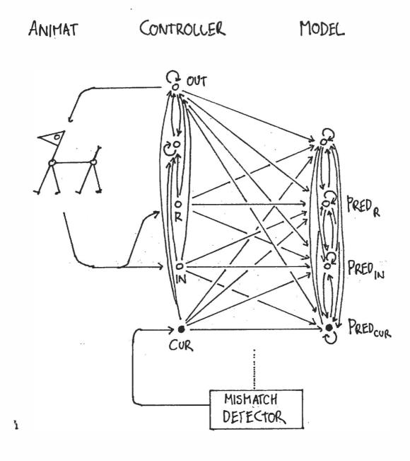
Figure 4: This figure is derived from figure 2. An additional reinforcement unit CUR for the control network gets activated by 'ideal mismatches' between expectations of the model network and reality. The model network needs an additional output unit  $(PRED_{CUR})$  for predicting CUR. It models its own ignorance, thus showing a rudimentary form of introspective behavior.
