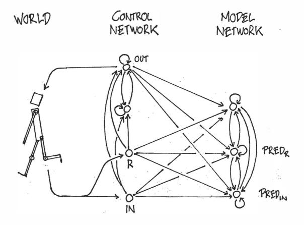
Figure 2: A control network with internal and external feedback is shown. For simplicity, only one normal input unit (IN), only one reinforcement input unit (R), only one hidden unit and only one output unit (OUT) are depicted. A model network (only one hidden unit is shown) is trained to simulate the environmental dynamics by predicting the control network's input (PRED\_{IN} and PRED\_R). The model hetwork provides credit assignment paths for the control network.
