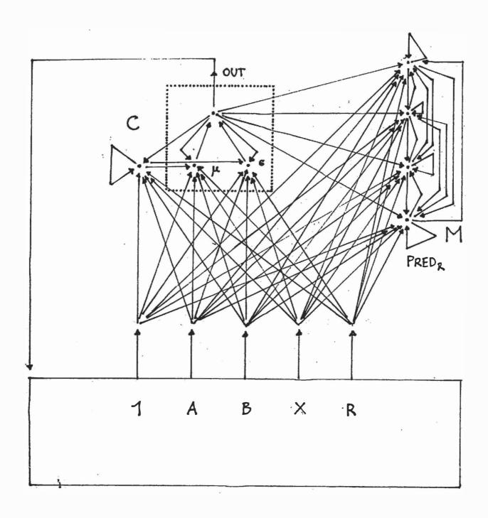
Figure 3: Topology of the controller/model combination for the flip-flop experiment. The block below represents the environment. The dashed line includes the sub-nodes for mean and variance generation for the controller's output unit.
