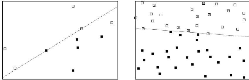
**Fig. 5.** Example scenarios with 10 (left) and with 50 (right) robots, after running the algorithm for 120 s. Black nodes indicate loaded robots, while white ones indicate unloaded robots. In each case, we draw the line that is found by the ILP in the evaluation of linear separability.
