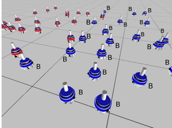
**Fig. 1.** Example of spatially segregated classes. Robots in class  $C_0$  show blue LEDs (a 'B' label is positioned beside each robot in class  $C_0$  to help readability also in greyscale), robots in class  $C_1$  show red LEDs (and have no text label).
