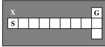
Figure 3.6: The T-Maze task. The agent observes its immediate surroundings and is capable of the actions goNorth , goEast , goSouth , and goWest . It starts in the position labeled ‘S’, there and only there observing either the signal ‘up’ or ‘down’, indicating whether it should go up or down at the end of the alley. It receives a reward if it goes in the right direction, and a punishment if not. In this example, the direction is ‘up’ and N , the length of the alley, is 8.
