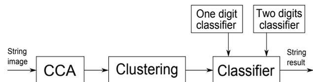
**Figure 1. Numeral string recognition system (CCA = connected component analyzer).**
