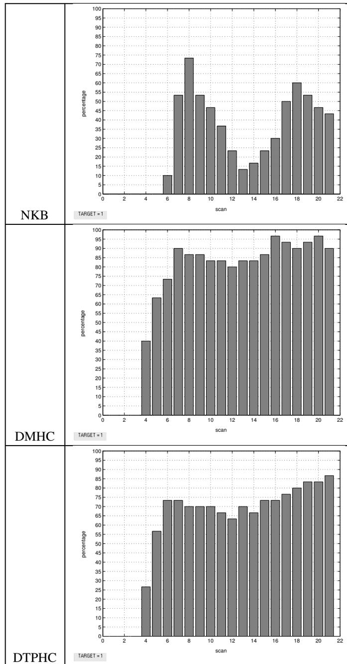
Fig. 10. Aircraft crossing the shore in a HC zone without maneuver: percentage of successful target tracks
