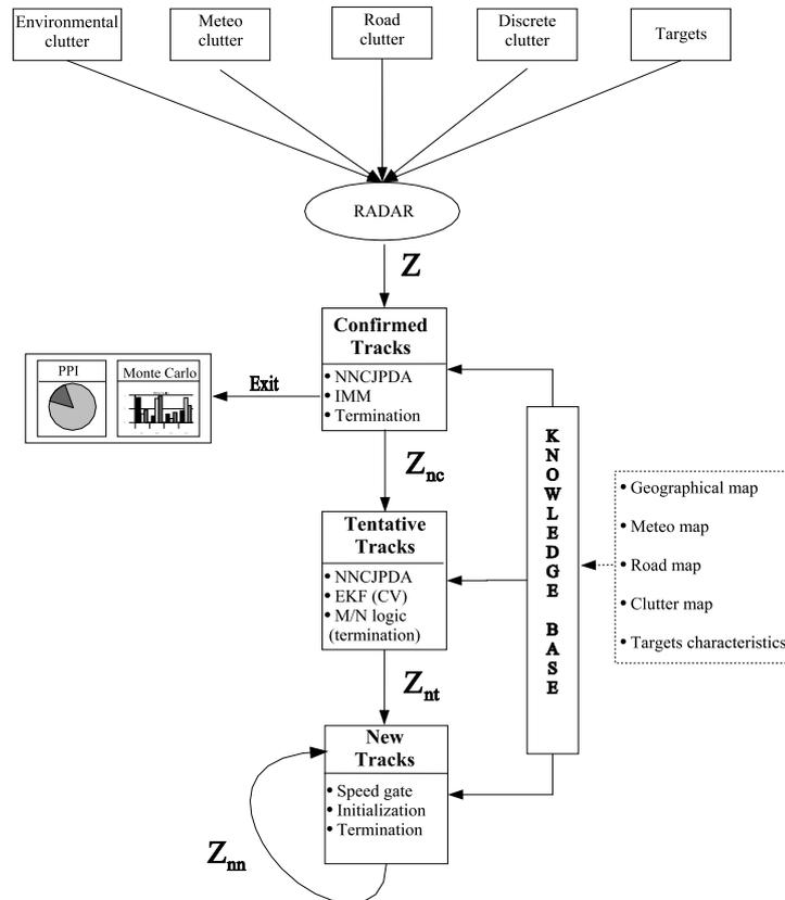
Fig. 3. Architecture of the KB tracking system
