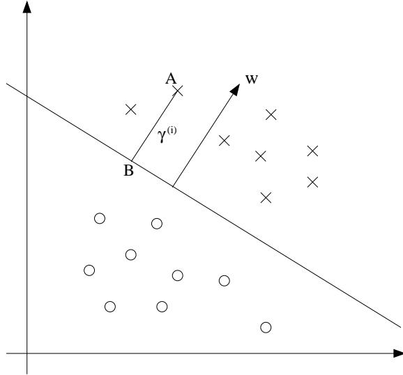
The decision boundary corresponding to  $(w, b)$  is shown, along with the vector  $w$ . Note that  $w$  is orthogonal (at  $90^\circ$ ) to the separating hyperplane. (You should convince yourself that this must be the case.) Consider the point at A, which represents the input  $x^{(i)}$  of some training example with label  $y^{(i)} = 1$ . Its distance to the decision boundary,  $\gamma^{(i)}$ , is given by the line segment AB.
